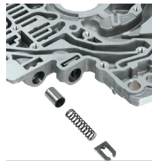
45RFE TCC Accumulator Spring Part No. 16 MP.52
